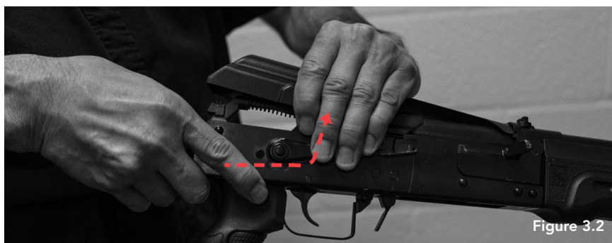
Figure 3.2 — Detaching The Receiver Cover
