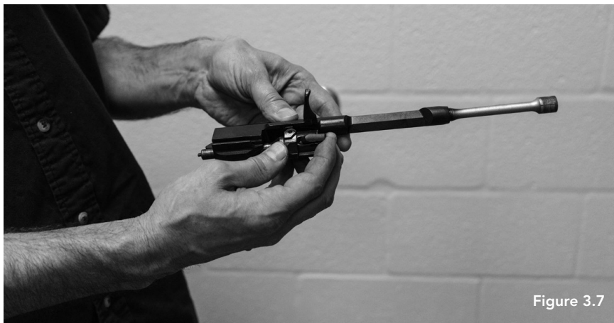
Figure 3.7 — Detaching The Bolt From The Bolt Carrier
