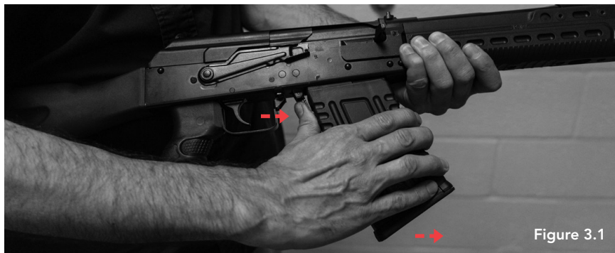
Figure 3.1 — Detaching The Magazine
