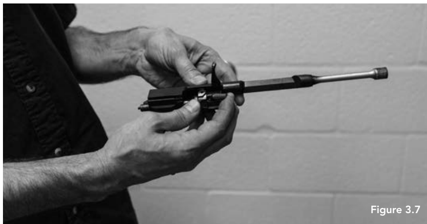
Figure 3.7 — Detaching The Bolt From The Bolt Carrier
