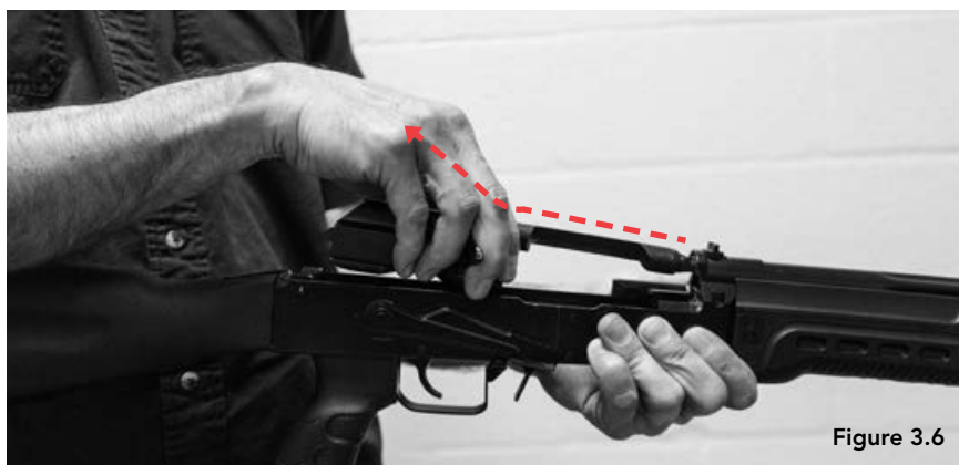
Figure 3.6 — Detaching The Bolt Carrier And The Bolt
