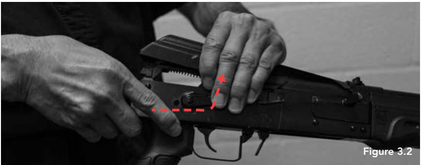
Figure 3.2 — Detaching The Receiver Cover
