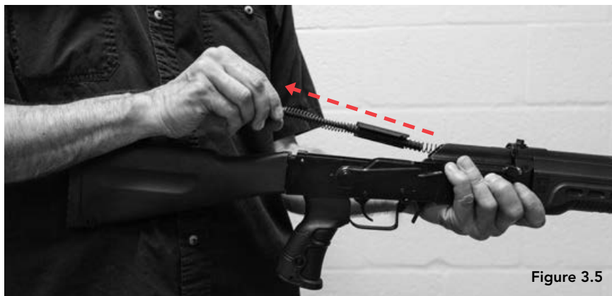
Figure 3.5 — Detaching The Recoil Spring Guide Assembly
