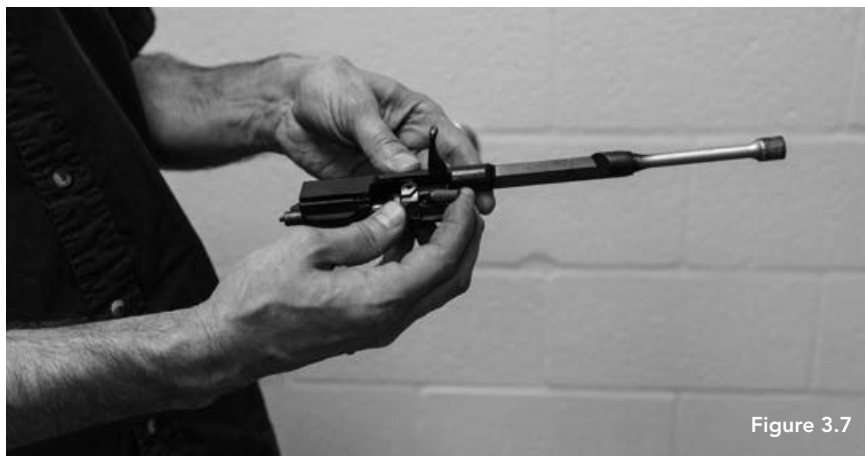
Figure 3.7 — Detaching The Bolt From The Bolt Carrier
