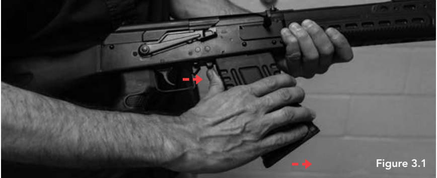
Figure 3.1 — Detaching The Magazine
