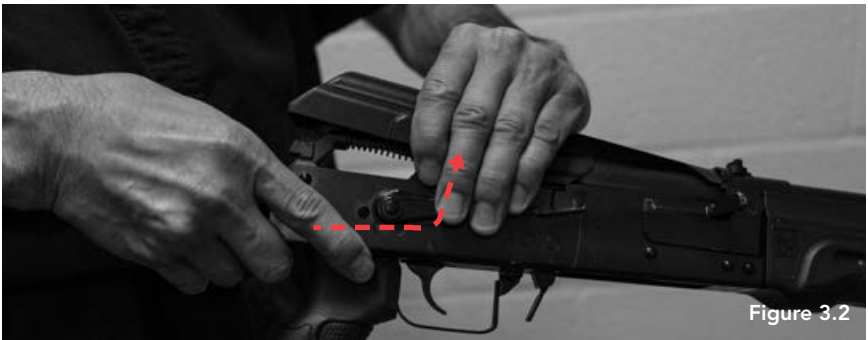
Figure 3.2 — Detaching The Receiver Cover
