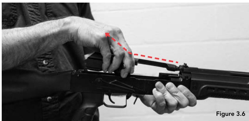
Figure 3.6 — Detaching The Bolt Carrier And The Bolt
