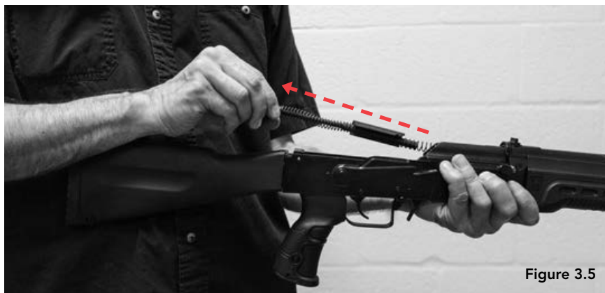
Figure 3.5 — Detaching The Recoil Spring Guide Assembly
